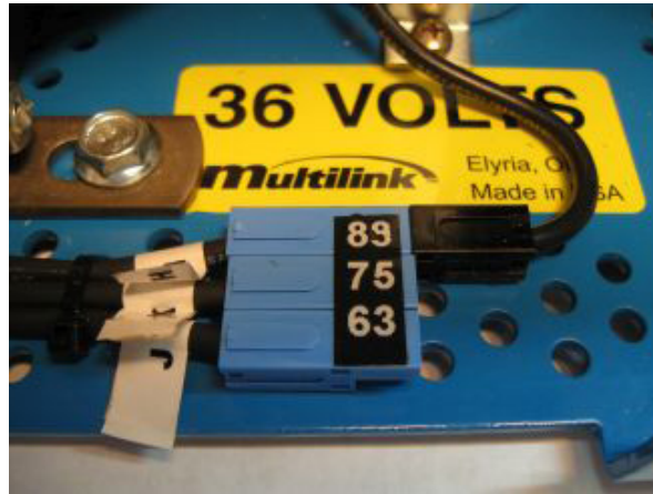
Fig. 4-2 Output Voltage Select Jumper Detail
